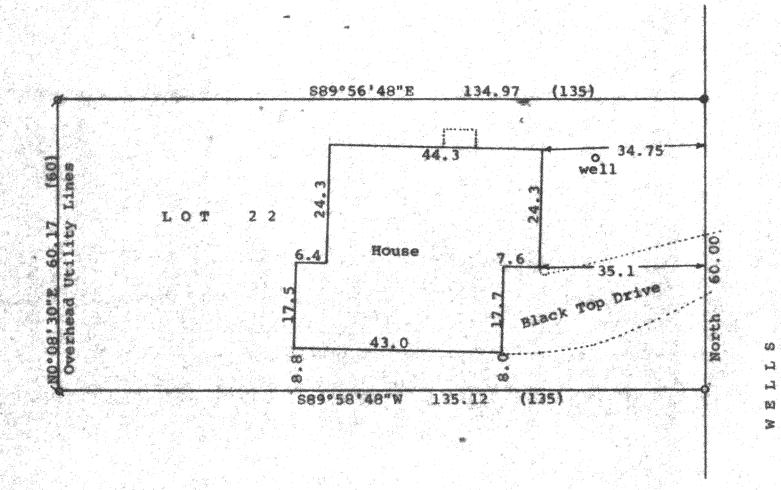
Scale - 1" = 20'  $\beta = 3/4$ " Iron Pipe Pound N= 13" Iron Pipe Found o = 1" Iron Pipe Pound down 1' ly" Iron Pipe Set over it at ground surface (0.00) = recorded distance
